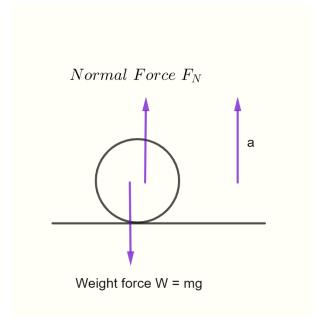
During the bounce (the instant the ball is in contact with the surface):
