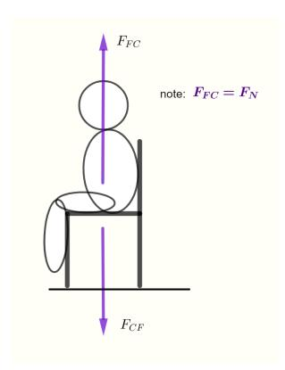
$F_{FC} = -F_{CF}$  where the negative sign indicates that these forces are acting in opposite directions. Recall your notes on vectors. The magnitude of the forces are equal but the direction is opposite.
